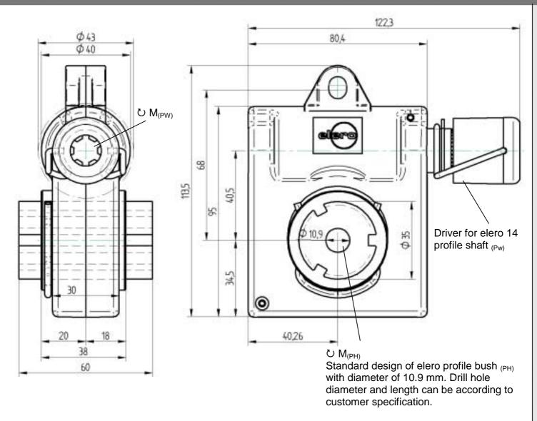
Materials: Housing and gear parts made from high-quality plastic elero 14 profile shaft (PW)
